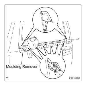
(b) Using a moulding remover, disengage the 8 claws and remove the front door glass outer weatherstrip.
